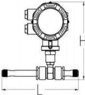
DN4-DN10 Threaded connection sensor (including straight pipe section)
