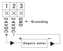
Ampere Meter Diagram of Two-wire
