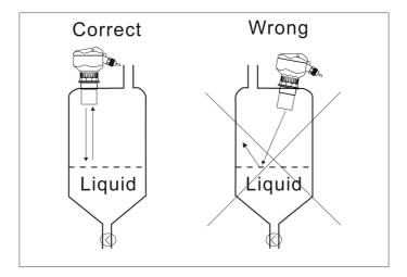
Sensor probe shall be perpendicular to medium surface
