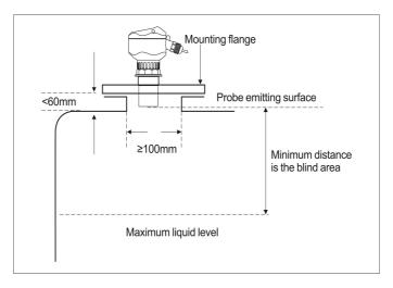
Flange installation in a short connecting pipe
