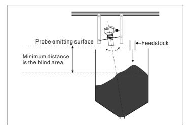
Integrated-type sensor - doorframe installation
