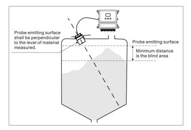
Remote-type sensor installed on container flange
