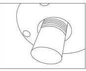
06.Place a spacer of the same inner diameter under the flange
