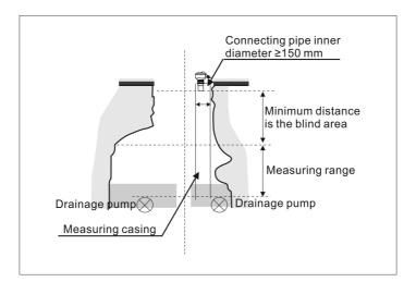
Connecting pipe and measuring casing used for drainage well measurement
