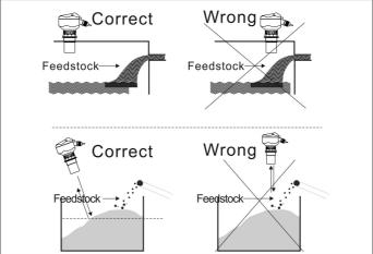
Sensor shall not be installed in or above the charging feedstock flow
