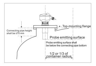
Installation on flange - arch tank top
