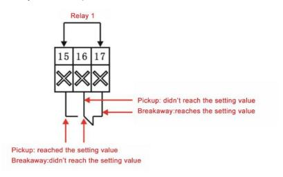
4.4.2. Wiring diagram of integrated-type:
