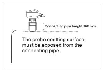
Probe installation on nipple joint
