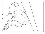
07.Tighten nuts to fix the transducer
