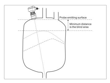
Integrated-type sensor - installation via nipple joint
