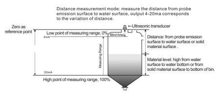
Fig. 1.1 Diagram of distance measurement
