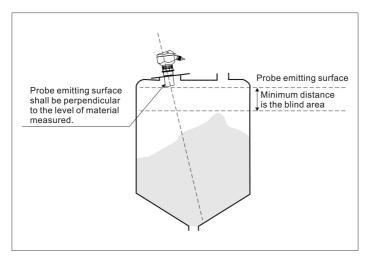
Integrated-type sensor installed on container flange
