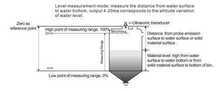
Fig. 1.2 Diagram of material measurement level
