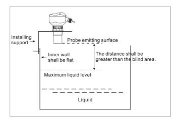
Installation on open container - with top against the support at one side
