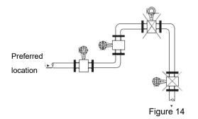
The pipe is routed to the highest point (Bubble accumulation in the measuring tube is likely to cause produce measurement errors!) Make sure the pipeline is always full.
