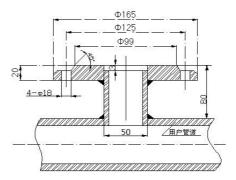
Figure 49 Welding of the mounting base
