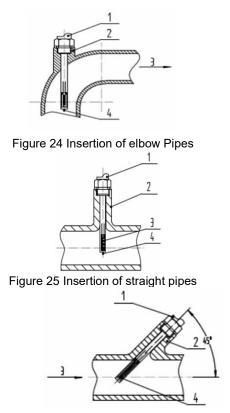
Figure 26 Insertion of sloped pipes
