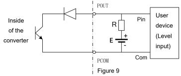
Recommendation: The pull-up resistor R in the figure is recommended to use a 2K, 0.5W resistor, and the power supply E is recommended to use 24V DC.
